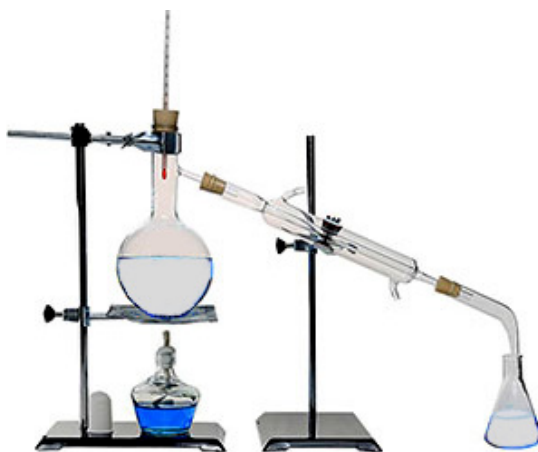
Figure 1. Simple distillation setup
